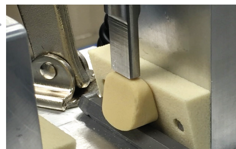
Figure 2. Instron mechanical tester setup with Sawbones and DPS-Evans-1812 Evans Osteotomy Wedge. This image depicts the Instron with the jaws apart to show the graft in place. The hex wrench is removed once the jaws are closed.
